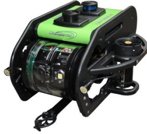
Figure 1: Seabotix LBV 300 Remote Operated Vehicle (ROV). This vehicle was used as a test target for the proposed system.
