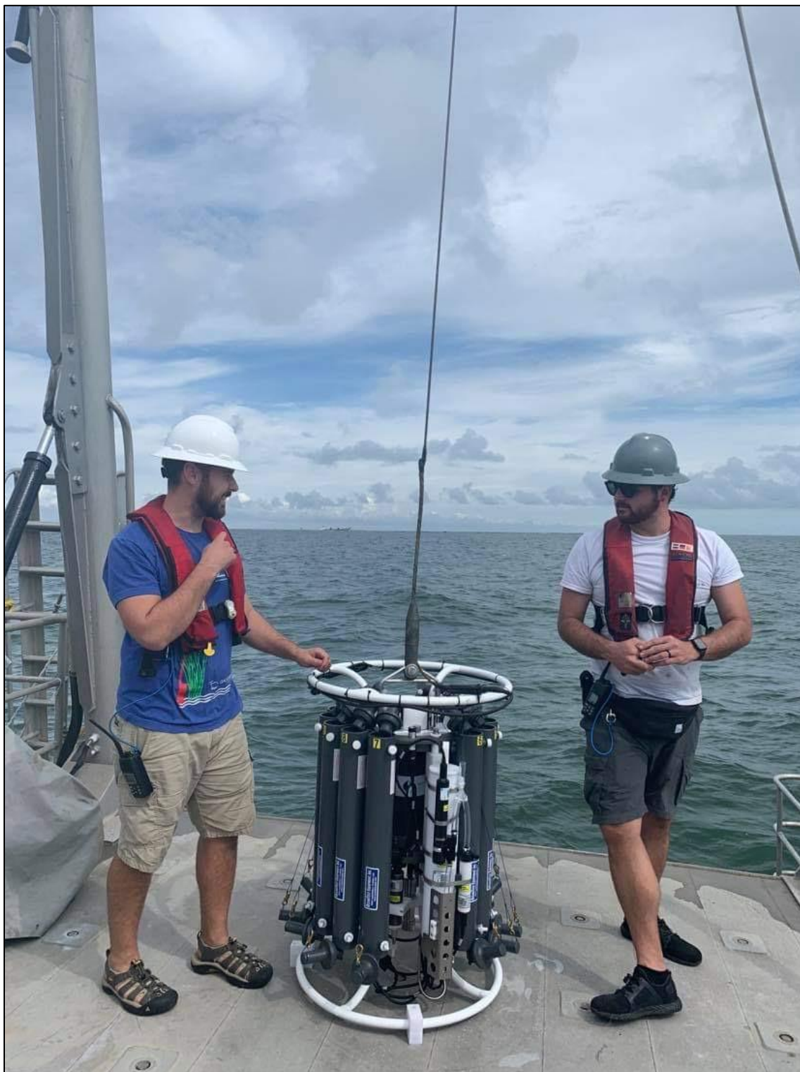
FGBNMS researchers prepare to deploy water sampling carousel aboard the R/V Manta . Photo: Emma Hickerson
