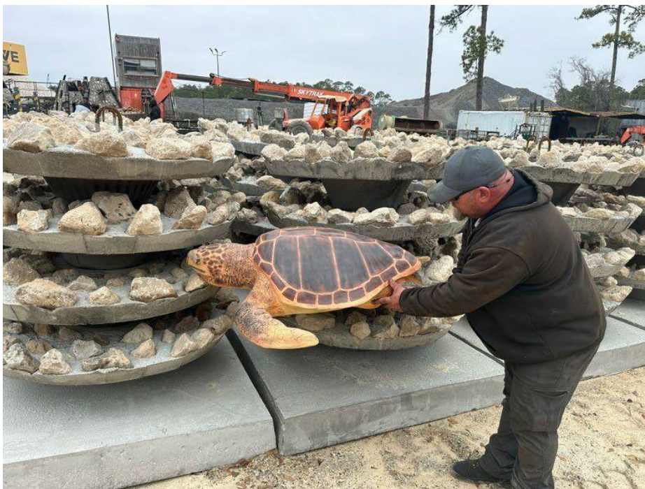
Figure 1. A photo (provided by the USACE) of the prefabricated Juvenile Reef Module made from limestone and oyster shell embedded discs mounted on a concrete cylinder that is embedded into a concrete slab. A model of an adult loggerhead is used to show the scale of the structure.
