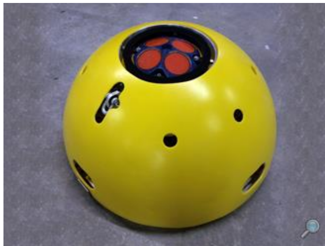
Figure 14. Mooring Systems, Inc. (MSI) H-TRBM-35 and H-TRBM-48 (formerly GP35 and GP48), which differ in diameter. The bottom mount holds an upward-facing acoustic Doppler current profiler (ADCP) and is lowered to the bottom to deploy and recovered with a grapnel that is dragged to snag the ground line connecting the mount to an anchor. Specifications for the mount of both sizes are here: https://www.mooringystems.com/mounts.htm (Image from MSI.)
