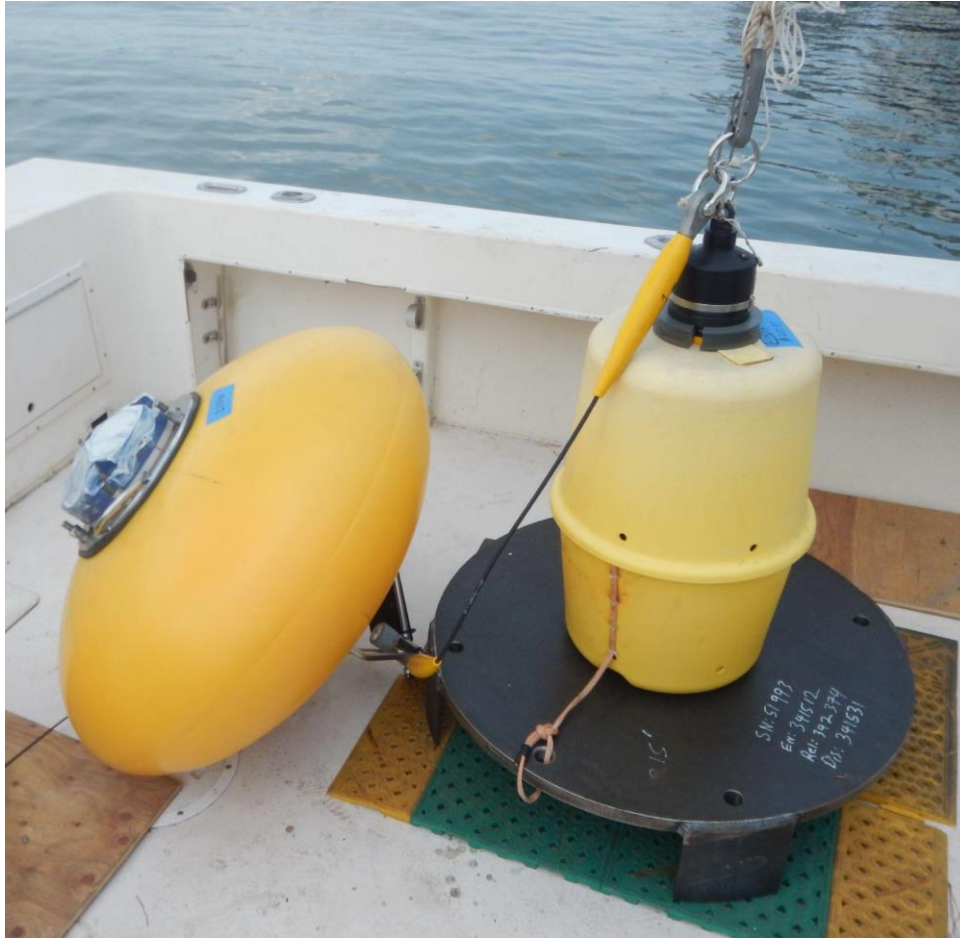
Figure 13. Subsurface ellipsoid acoustic Doppler current profiler (ADCP) buoy (SEABY). The ellipsoid buoy holds the upward-facing ADCP and is attached to the acoustic release and anchor system with a taut wire line.
