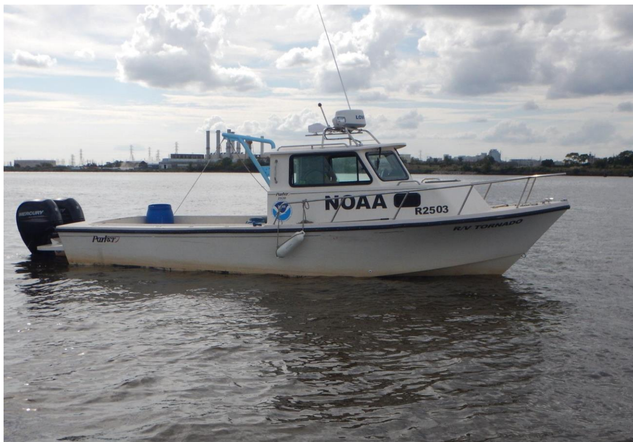
Figure 9. The NOAA R/V Tornado (7.6-meter [25-foot] Parker) equipped with a davit used for operations in the Delaware Bay and River.
