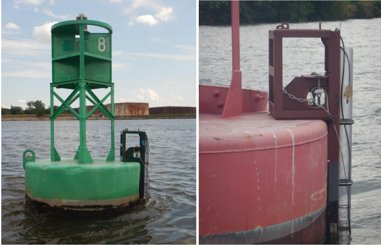
Figure 17. Clamparatus on a green (left) and red (right) aid to navigation (ATON).
