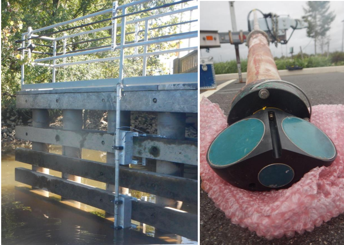
Figure 16. Bridge cribbing side-looking mount (left). Side-looking acoustic Doppler current profiler (ADCP) deployed in the bridge cribbing mount (right).
