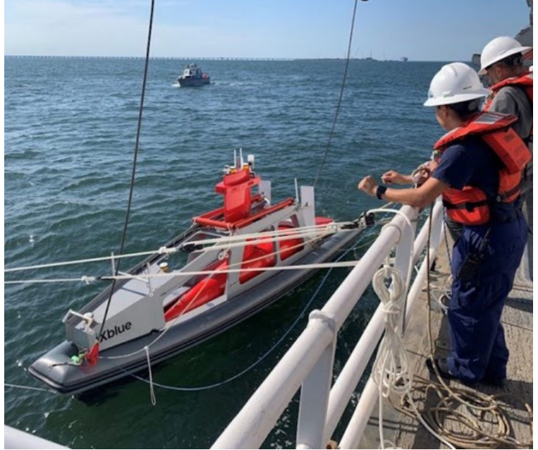
Image 5: A DriX uncrewed surface sits in its docking station alongside the NOAA Ship Thomas Jefferson. Photo: NOAA
