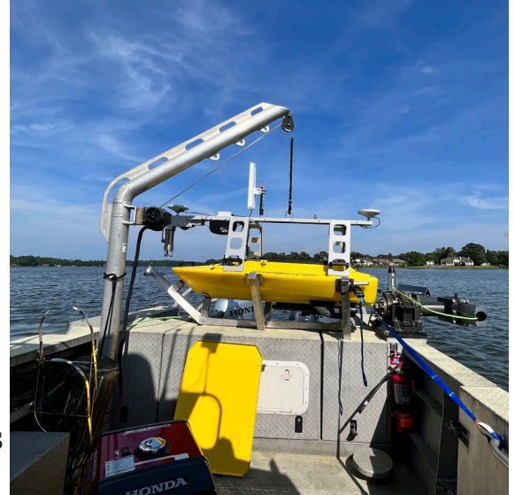
Image 3: An EchoBoat UMS on the stern of a survey vessel before deployment. Photo: NOAA
