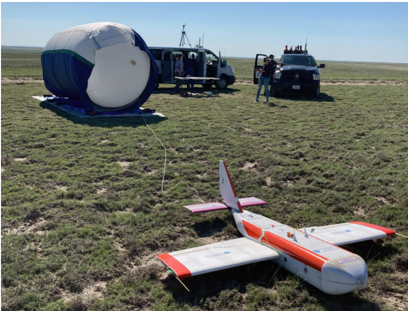
Image 13: The HORUS glider and balloon prepared for a test flight in Colorado's Pawnee National Grasslands. Photo: NOAA
