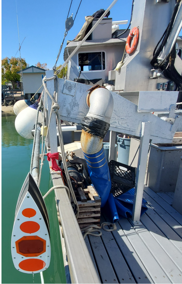
Figure 6: Transducer locations on the bottom of the pole-mounted multi-transducer array (MTA4) installed on the F/V Long Beach Carnage .
