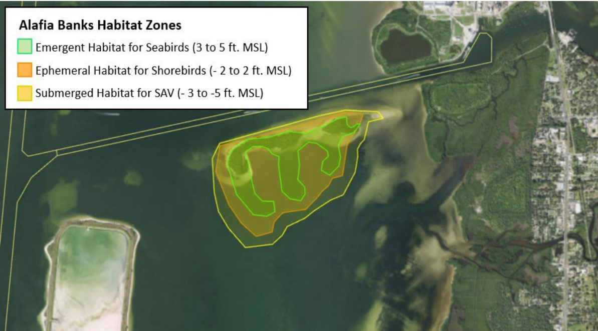
Figure 7. Conceptual design of the proposed habitat zones that would be created using dredged materials at the Alafia Banks Critical Wildlife Area.
