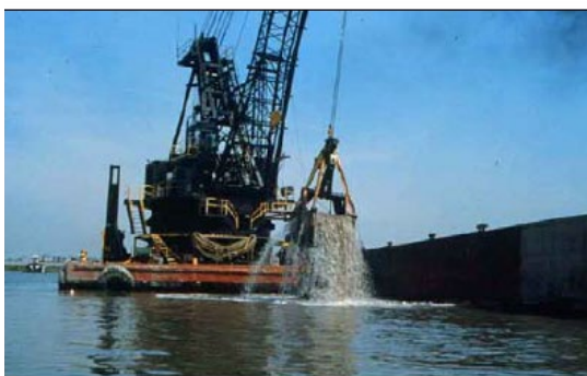
Figure 8. Mechanical dredge (clamshell bucket and barge).
