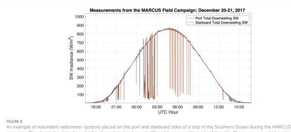
An example of redundant radiometer systems placed on the port and starboard sides of a ship in the Southern Ocean during the MARCUS field campaign. The dips in the data show shading from ship structures at different times on either side of the ship. The measurements have been tilt-corrected using the method described in Section 3.2.
