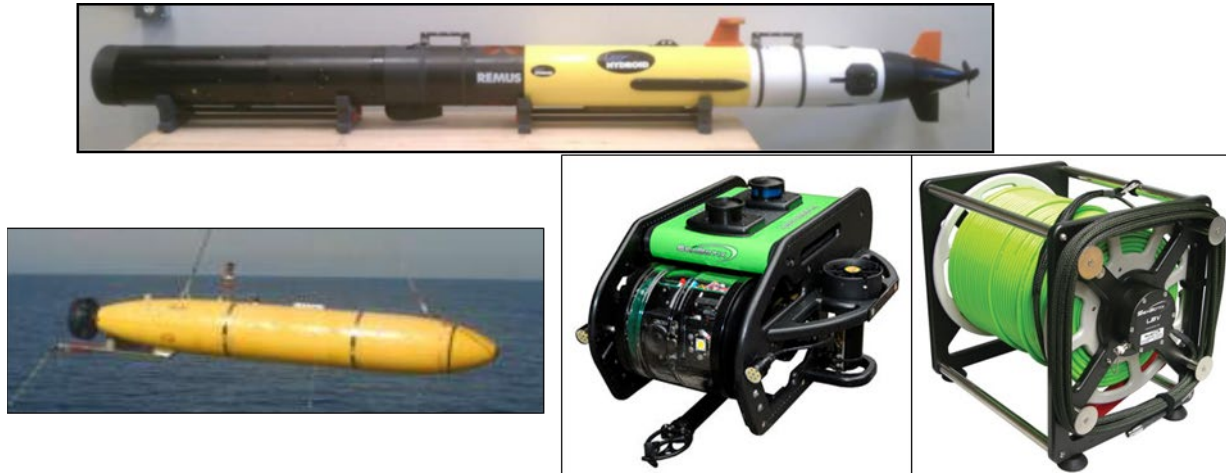
Figure 5. Examples of Unmanned Underwater Vehicles. Top panel is a Remote Environmental Monitoring Unit System 100; bottom left is a 21” Bluefin; bottom center is a Little Benthic Vehicle (LBV) 300; bottom right is the tether associated with the LBV300, resulting in a Tethered, Hovering Autonomous Underwater System.
