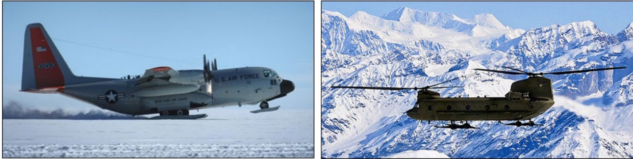
Figure 4. Examples of Military Fixed-Wing Aircraft (left panel; C-130) and Rotary-Wing Aircraft (right panel; CH-47) that may be Used During ICEX.
