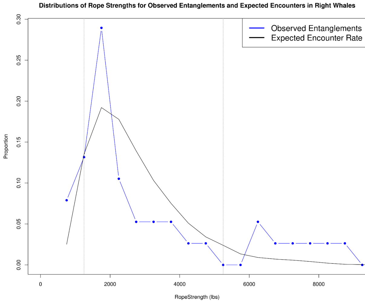
Figure 35. Distributions of rope strengths expected to be encountered by North Atlantic right whales ( Eubalaena glacialis ) in comparison to observed entanglements shows a similar trend with heaviest ropes more common in entanglements than expected.
