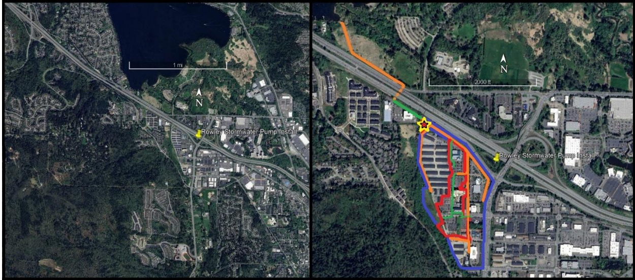
Figure 1. Google Earth images of the Hyla Crossing project site in Issaquah, Washington. Lake Sammamish is visible north-northwest of the project site, and the intersection of SR 900 with I-90 is to the east. The total stormwater catchment area is outlined in blue, with the Phase 1 catchment area outlined in red, and the pump station indicated by the star. Excavation areas for new pipelines are shown in orange, and project-related existing pipes are shown in green.
