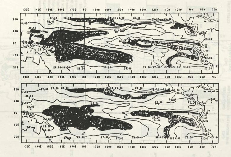
Figure 1. Upper panel: Model estimate for sea surface temperature for January 1988 after a 30 day integration with no corrections with in situ data. Lower panel: The field in the upper panel modified through the use of BSST and XBT information.
