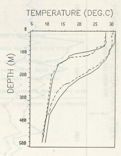
Figure 8. Comparison between two XBT profiles collected in January 1988 and the model thermal fields, without assimilation of data for this month, interpolated to these XBT locations. Dashed curves are the XBTs. Much of the XBT editing is automated, with the model fields being used for reference. These two profiles were identified by the editing procedures as being outside the norm and requiring human attention.
