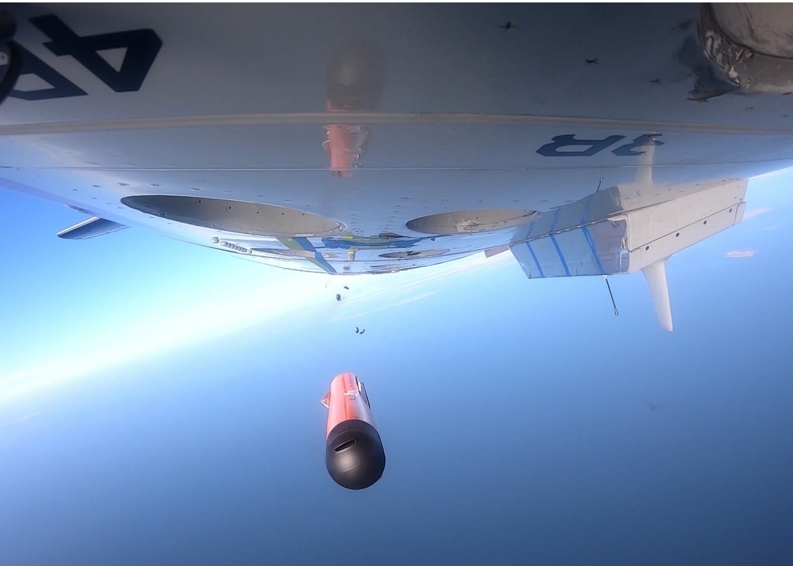
Image 4: The Anduril Altius-600 UAS is deployed from a NOAA hurricane hunter aircraft. Photo: NOAA
