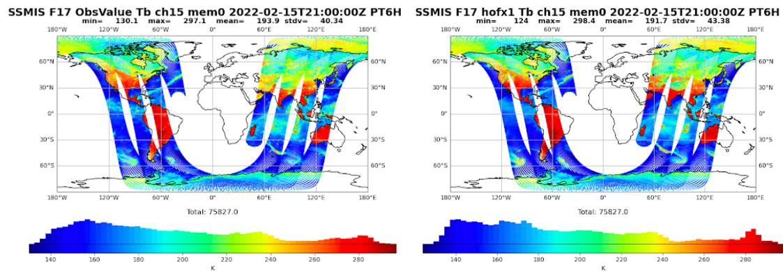
*Observed (left) versus CRTM simulated (right) brightness temperatures for SSMIS Channel 15. See <https://skylab.jcsda.org/> for more visualized data across multiple sensors and time frames.*
