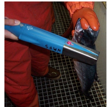
Figure 9 Scanning salmon for presence of CWT
