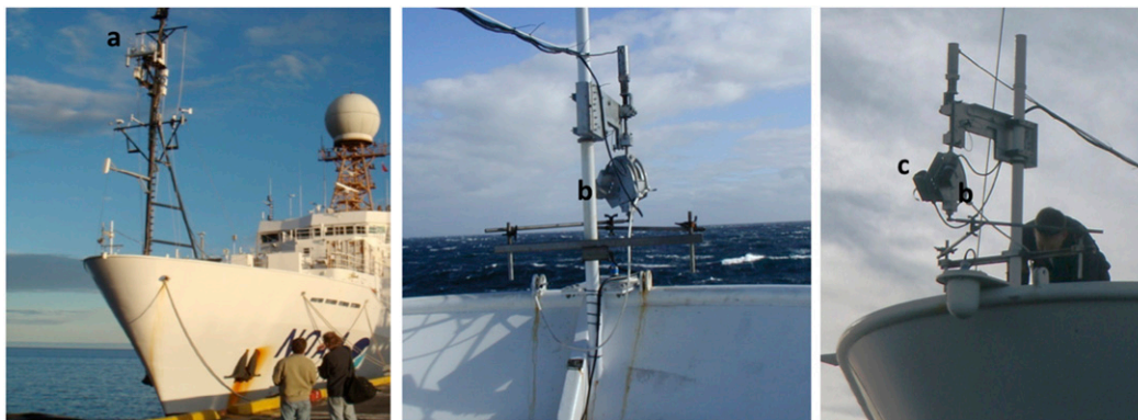
FIG. 4. The three radiometric sensors deployed during SO GasEx: (a) a downwelling irradiance sensor mounted on the top of the jack staff at 18 m, and (b) down-looking and (c) sky-viewing radiance sensors deployed at the bow. The downwelling irradiance and sky radiance signals are used as ancillary data and are not required in retrieving whitecap quantities. Proper viewing angles were maintained using a computer-based system that calculated the sun's azimuth angle relative to the ship and adjusted the position of the detectors using a stepping motor. A new version of this design is now available commercially (Sea-Bird/Satlantic).
