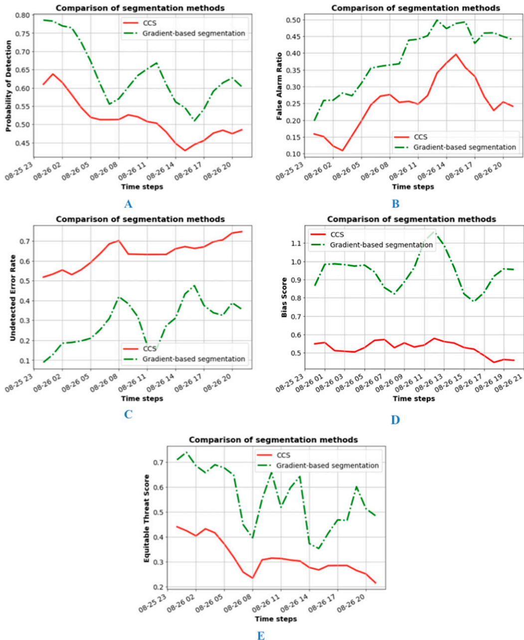
FIG. 10. Statistical comparison of two different segmentation algorithms for the Hurricane Harvey case: (a) POD, (b) FAR, (c) undetected error rate, (d) bias score, and (e) equitable threat score.
