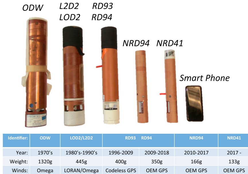
FIG. 2-4. History of dropsondes developed at NCAR. A smart phone is included for a size reference. © 2018 UCAR.
