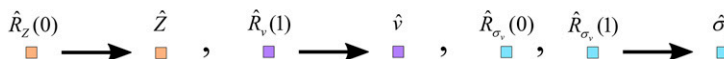
FIG. 1. Graphical depiction of the efficient implementation of adaptive pseudowhitening processing. Only the steps to produce the single-polarization spectral moments are included for simplicity.
