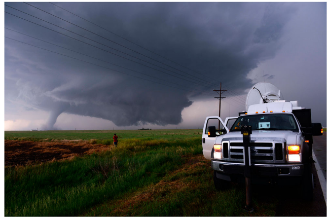
Fig. 9 RaXPoL, a rapid-scan, X-band, polarimetric mobile Doppler radar scanning a tornado in Kansas in 2016. Courtesy of H. Bluestein.
