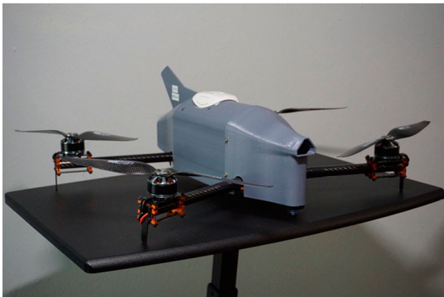
Fig. 10 CopterSonde UAS for atmospheric measurements made by the Center for Automated Sensing Systems at the University of Oklahoma. Photo courtesy of Tony Segalés.
