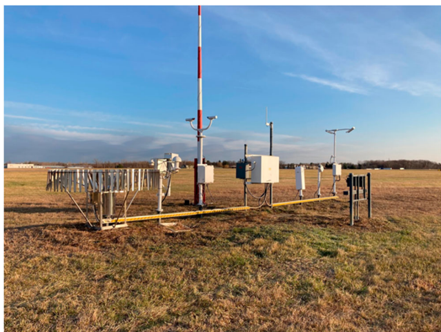
Fig. 8 Typical Automated Surface Observing System (ASOS). Courtesy of Kenneth Boutin, National Weather Service.
