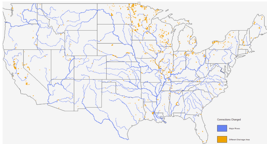
Fig. 9. Shows locations where total drainage area is more than 10% different from the NHDPlusV2 (McKay et al., 2015) and the reference flow network (Blodgett 2023-1). This comparison uses dendritic total drainage area assuming 0 drainage area at the top of any secondary (diverted) flowline. Note that the absence of yellow overlay indicates agreement in total drainage area.
