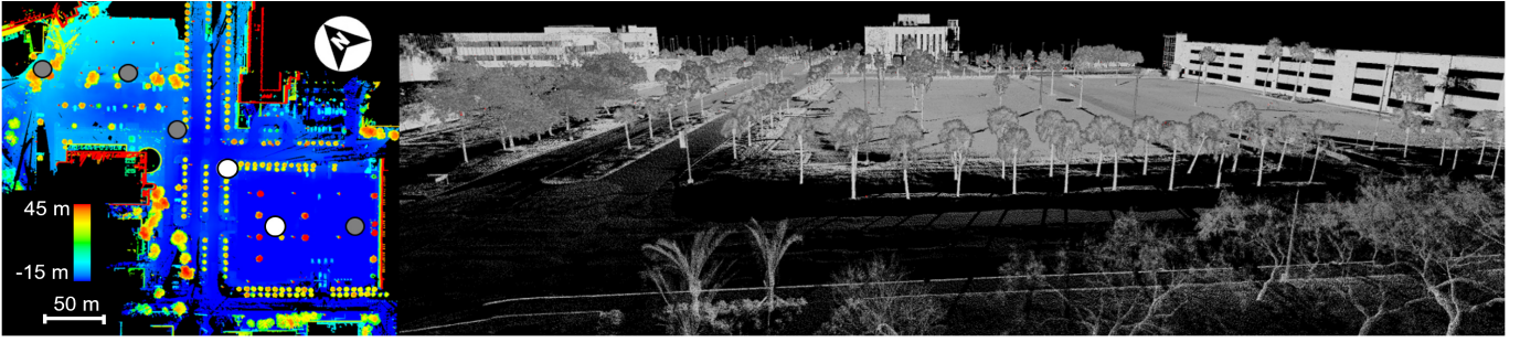
Fig. 1. Co-registered TLS point cloud of the campus. Side view is colored gray by reflectance. (Left) Top view is color-coded by height. Circles show six TLS positions in the October survey. White circles represent two TLS positions for the July survey.
