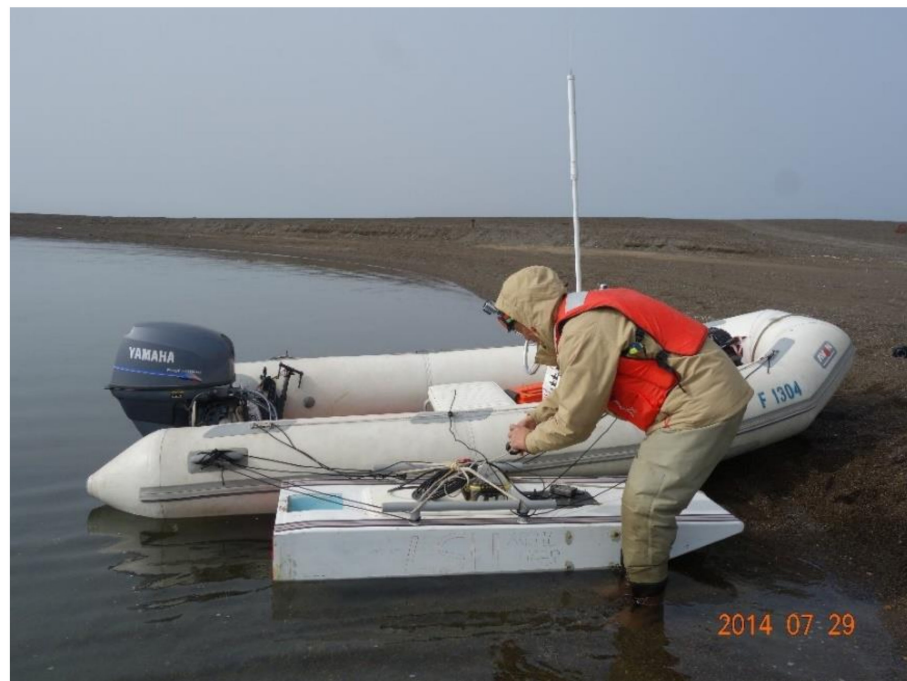
Figure 3. The inflatable vessel used to tow the fiberglass surface craft (in front of the inflatable vessel), which carried the M9 ADCP.
