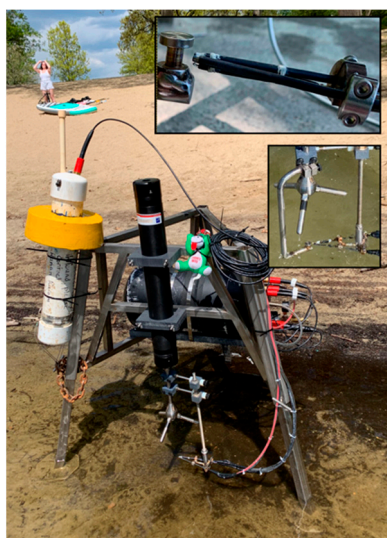
Figure 1. Eddy flux instrument mounted on benthic lander. Communication buoy, shown strapped to the lander for very shallow deployments, floats free for deeper deployments. ( Top inset ) FACT sensor head including optical fibers, conductivity electrodes, and thermistor. ( Bottom inset ) FACT sensing head shown with jig for aligning sensing volumes.
