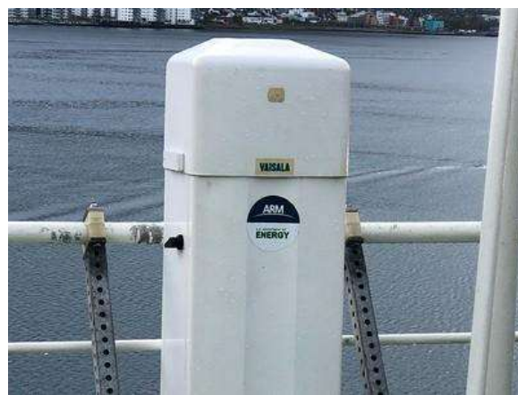
Figure A7. DOE ARM Ceilometer. [Image courtesy of the U.S. Department of Energy Atmospheric Radiation Measurement (ARM) user facility].
