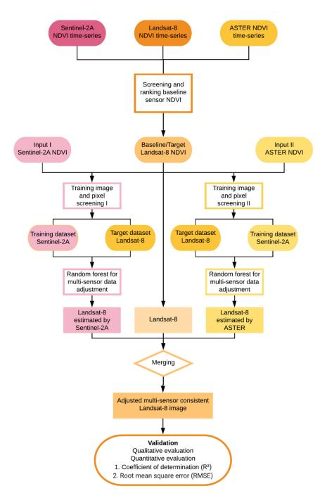
Figure 4. Schematic flowchart of the virtual constellation process.
