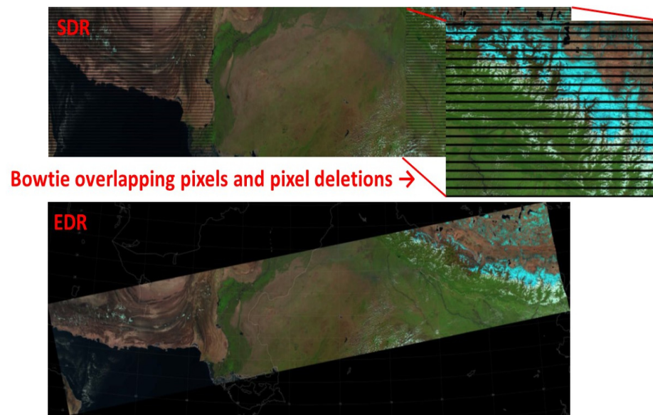
Figure 1. The difference between VIIRS SDR ( top ) and EDR ( bottom ) granules is the remapping into the GTM grid, which eliminates both the missing pixels (black lines at each end of the SDR granule) and also compensates for any remaining overlap in the SDR pixels.
