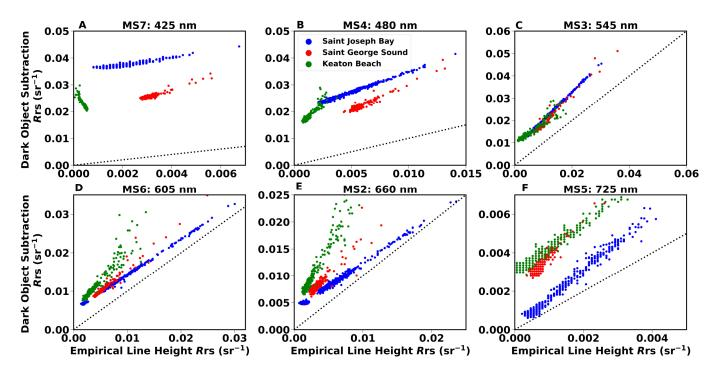
**Figure 5.** Comparison between  $R_{\rm rs}$  retrieval for ELH and DOS atmospheric correction for WV-2 bands MS2 through MS7. Data for each site are indicated by symbol color. Dotted line represents the 1:1 line of perfect agreement. Data consist of 300 randomly chosen points from each site, 100 from seagrass, 100 from submerged sand, and 100 from deep water.
