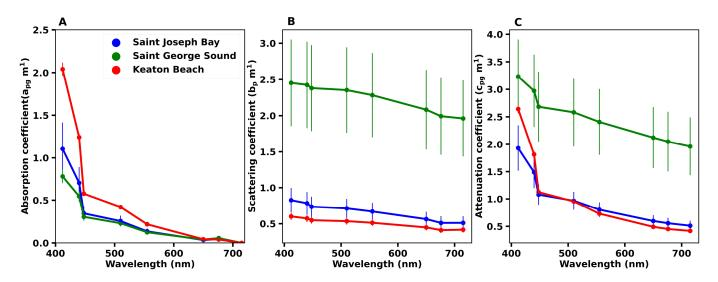
**Figure 4.** Mean spectra for (**A**) absorption ( $a_{pg}$ ), (**B**) scattering ( $b_p$ ), and (**C**) beam attenuation ( $c_{pg}$ ) coefficients measured using Sea-Bird/WetLabs ac-9 instrument in Saint Joseph Bay, Saint George Sound, and Keaton Beach. Error bars indicate  $\pm 1$  standard error of the mean for each wavelength bin.
