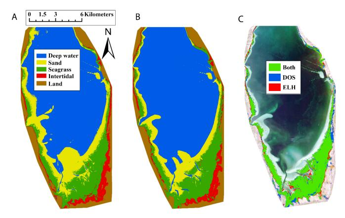
**Figure 6.** Habitat classification maps for Saint Joseph Bay using (**A**) ELH atmospheric correction and (**B**) DOS atmospheric correction. Habitat class is indicated by color identified in the legend in (**A**). (**C**) Comparison of pixels identified as seagrass using ELH and DOS atmospheric correction. Pixels mapped in green were identified by both. Pixels mapped in blue and red were identified only by DOS and ELH, respectively.
