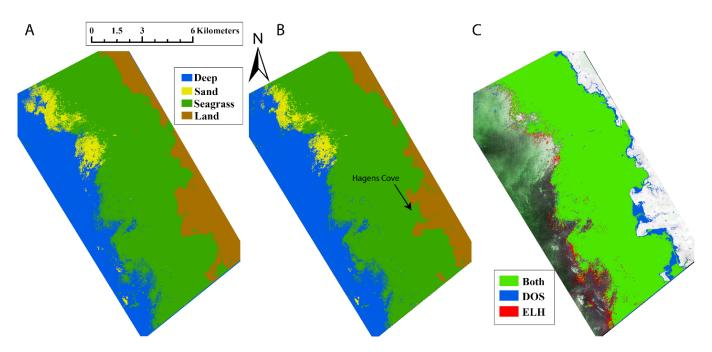
**Figure 8.** Habitat classification maps for Keaton Beach using **(A)** ELH atmospheric correction and **(B)** DOS atmospheric correction. Habitat class is indicated by color identified in the legend in Figure 6A. **(C)** Comparison of pixels identified as seagrass using ELH and DOS atmospheric correction. Pixels mapped in green were identified by both. Pixels mapped in blue and red were identified only by DOS and ELH, respectively.
