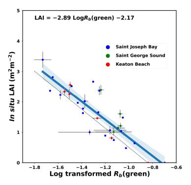
**Figure 9.** In situ measurements of  $R_b$ (green) and leaf area index from all three study sites. LAI values are averaged from randomized sampling within 20 m of a central location and are shown with  $\pm 1$  standard error bars.
