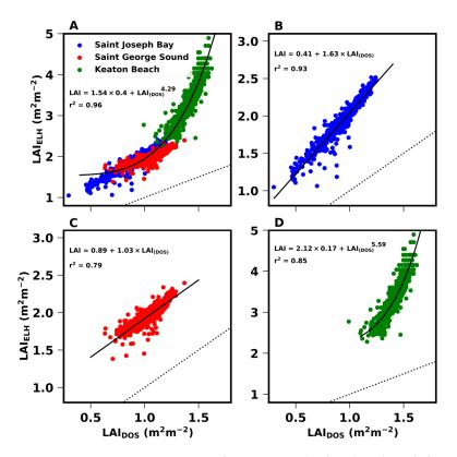
**Figure 14.**  $LAI_{(DOS)}$  versus  $LAI_{(ELH)}$  from 1000 randomly selected pixels from each site. (**A**). All sites combined. (**B**). Saint Joseph Bay. (**C**). Saint George Sound. (**D**). Keaton Beach Dotted line represents the 1:1 line, and points above this line are higher in the  $LAI_{(ELH)}$  retrieval.
