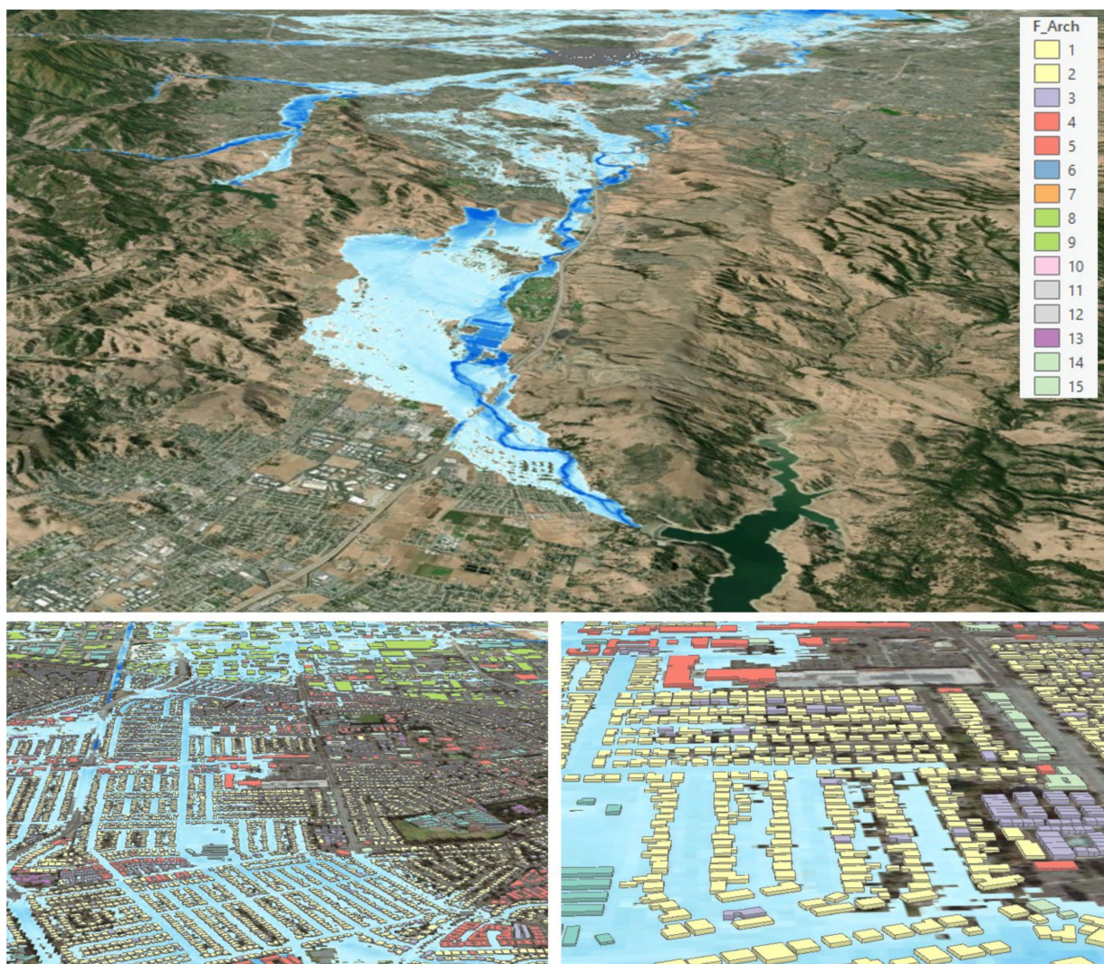
Figure 13. A 3D view for the Santa Clara County with buildings color-coded based on their archetypes and overlaid with the flooding (hazard) layer to identify the exposed buildings with close-up views on one of the flooded locations.
