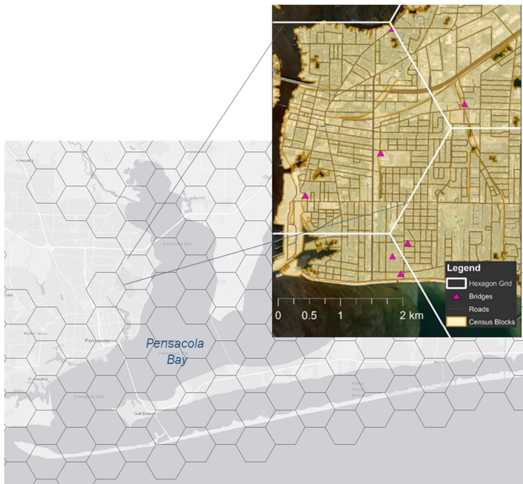
Figure 2. Hexagon grid used for data summaries. Here is an example of the different geometries of damage/impact data, including Census block polygons, roads represented by lines, and bridges represented by points. The values are summarized to a 10 sq. km hexagon grid.
