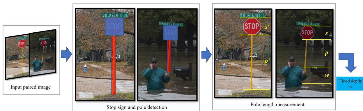
Fig. 6 Workflow for estimating flood depth in a sample paired pre- and post-flood photos (base post-flood photo is courtesy of Erich Schlegel/ Getty Image)
