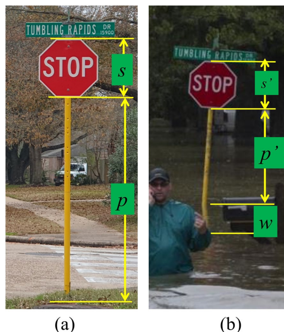
Fig. 1 Flood depth estimation in a paired a pre-flood photo and b post-flood photo (base photo in b ) is courtesy of Erich Schlegel/ Getty Images)
