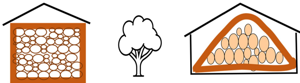
Fig. 14 Baby Vault is a small shelter that can be built manually or with light machinery, using wood sourced from the immediate vicinity. The enclosure can be constructed with traditional adobe technique using local material of mud and straw. An underground version is also possible. Version Baby1 (Left) constitutes vertical walls that may be constructed before filling in logs, while Version Baby2 (Right) piles up logs naturally first before covering with mud or clay
