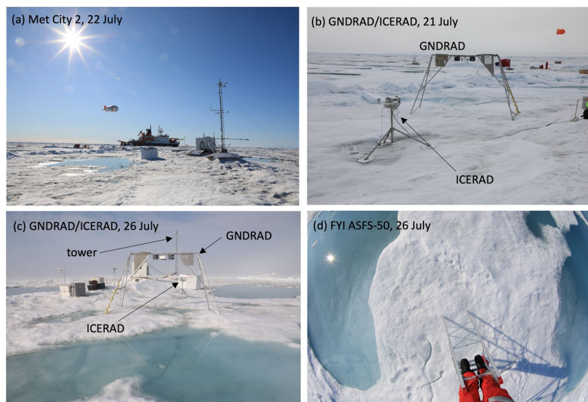
Fig. 7 Met City 2 during Leg 4. (a) Tower and nearby installations at Met City 2 on 22 July. (b,c) ARM ICERAD/GNDRAD systems during period of expansion of melt ponds. (d) Wide-angle photograph of the surface beneath the ASFS-50 boom at First Year Ice (FYI) on 26 July.
