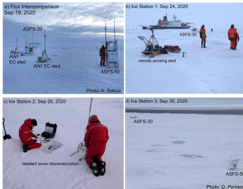
Fig. 10 Special measurement periods with the ASFS at the end of Leg 5. (a) A turbulent flux intercomparison period was conducted on 19 September between the ASFS and the AWI flux sleds. (b,c,d) three ice stations were conducted during the return transit using ASFS along transects to measure the spatial variability of the energy fluxes and obtain independent estimates of emissivity. These were done in conjunction with measurements by the cryospheric and remote sensing teams along identified transects.
