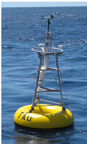
Figure 6. NOAA TAO buoy similar to those hosting RIO GPS receivers in the Pacific Ocean.
