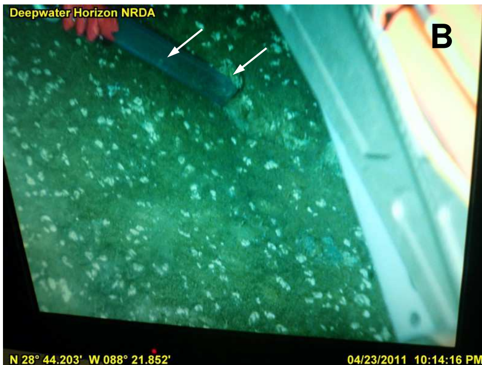
Fig. 5. Photographs of the seafloor impacted by SBM. (A) representative photograph of ubiquitous SBM coverage manifest as white “stars” protruding from a subsequently deposited layer of flocculent material observed along transects FP-0 and FP-1 (Fig. S-1) and (B) close-up showing slurrp gun nozzle being used to vacuum white material (arrows). This photo shows collection of a nearly pure SBM sample (HSW2L2_FP0094_B0423_W_1543_50_P_W_870) shown in Fig. 6. Photographs of live ROV video monitors by JRP.
