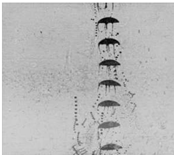
Figure 2. Dispersed oil droplet shedding microdroplets while rising. (Image used with permission from David Murphy and Cheng Li, Johns Hopkins University).
