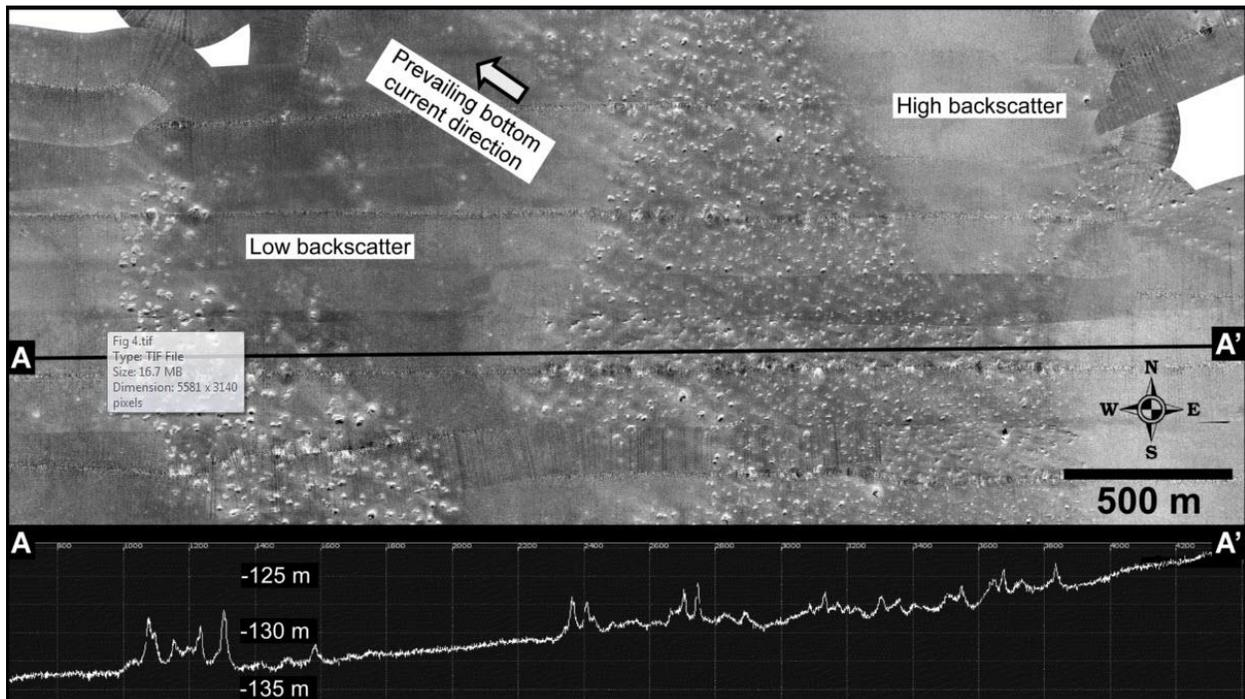
Fig. 4. A closer view of backscatter showing the noticeable variation in intensities attributed to surface sediment grain-size variation. A-A' is a water depth profile from the co-registered swath bathymetry data. Streaks of lighter intensity (coarser sediment) suggest net bottom-current transport of coarse-grained sediment (production and bioerosion) to the NW. Dark shades are lower backscatter and shadows. Location in Fig. 3.
