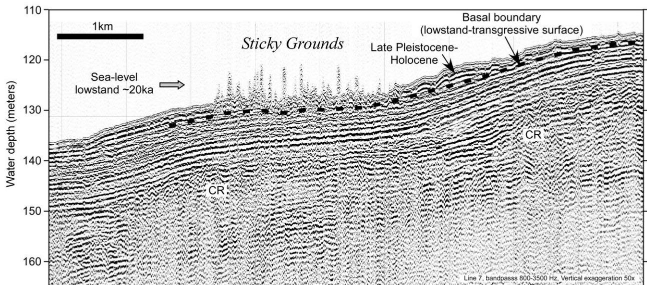
Fig. 2. Boomer seismic profile showing location of carbonate mounds between 120 and 130 m water depth. This dip-orientated profile shows the mounds in this area are restricted to a zone parallel to bottom contours and a flattened slope gradient. Chaotic reflections (CR) may indicate
