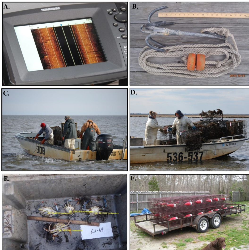
Fig. 4. A. Humminbird 898C SI Combo Side Imaging Sonar/External GPS unit used by commercial partners for re-acquisition of DFG targets and in-season recoveries. B. 2–4 kg single grapple used for shallow water DFG recoveries from silt/mud habitats. C. Example of typical industry vessel (< 8 m length, shallow draft, limited hauling capacity) used for shallow water DFG recoveries. D. Successful DFG recoveries after mud and silt removed. E. Bycatch photograph example with 3 blue crabs, 1 rock crab, metric ruler, trap ID (KU-64), and Image Pro overlay shown. F. Refurbished recovered traps ( n = 39 ) worth $1560 ($40 each). (For interpretation of the references to color in this figure legend, the reader is referred to the web version of this article.)
