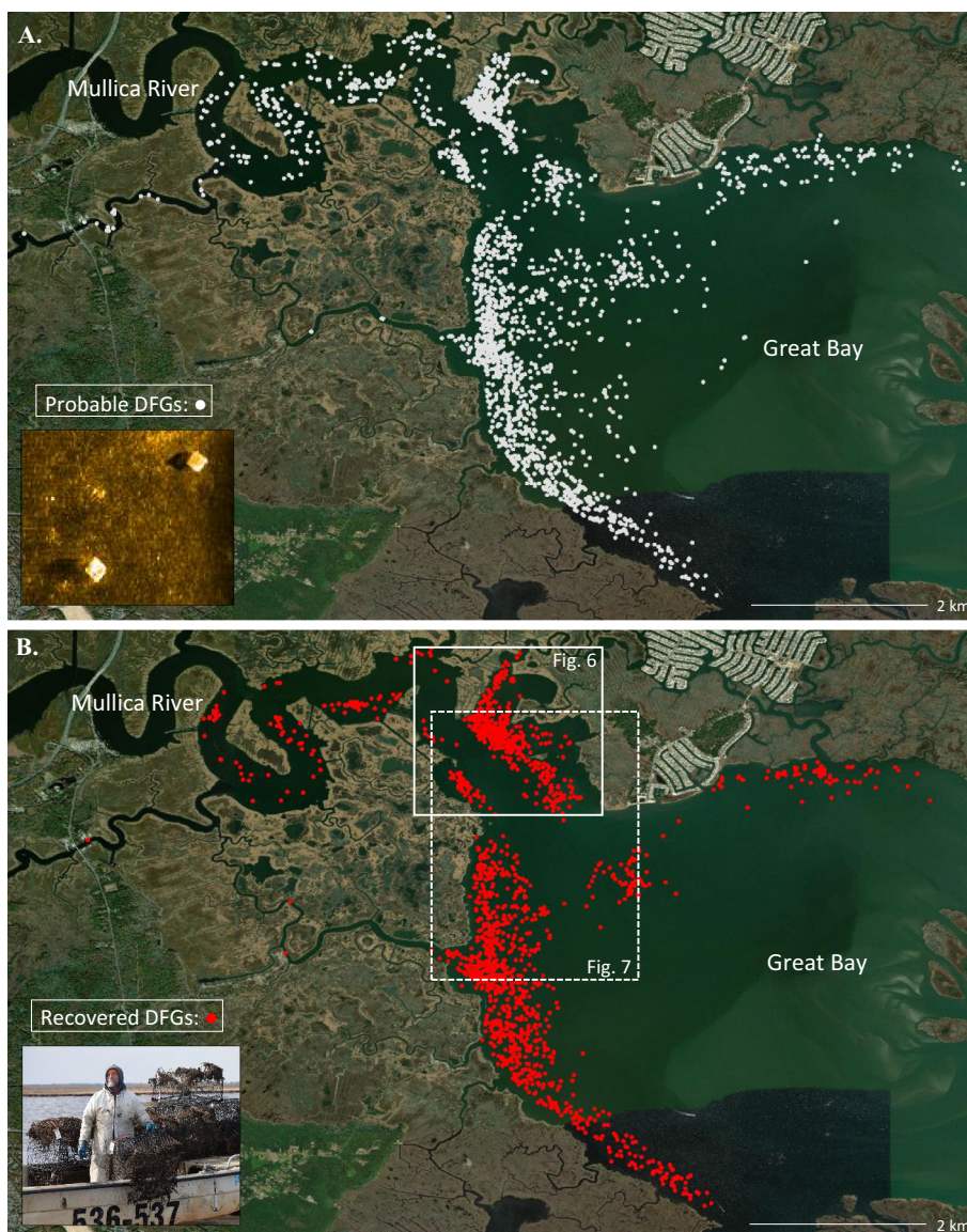
Fig. 5. A. Probable DFGs (white circles) in MRGB from scientific grade side scan sonar surveys. B. Recovered DFGs (red circles) in MRGB. White, solid rectangle denotes area detail in Fig. 6. White, dashed rectangle denotes area detail in Fig. 7. (For interpretation of the references to color in this figure legend, the reader is referred to the web version of this article.)
