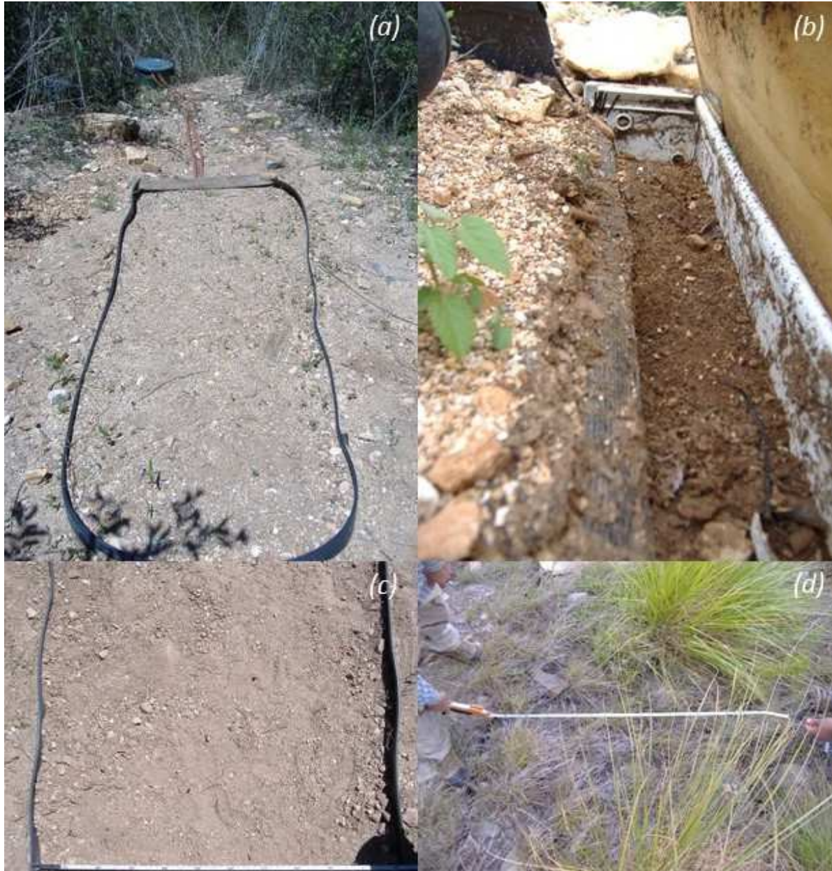
Figure 2. Pictures showing (a) bounded plot with Gerlach trough layout and collection containers, (b) detail of a Gerlach trough with fabric, (c) a disturbed plot surface, and (d) an undisturbed plot surface.
