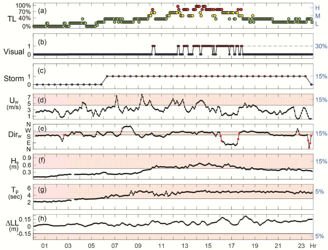
Fig. 8. Likelihood of flash rip hazards on July 12, 2017: (a) total likelihood (TL) ranging from 0 to 100%, and the three tiers of risk in high (red), moderate (yellow), and low (green); (b) image observation factor, with 1 (red) for flash rips detected in the image and 0 (blue) otherwise; (c) storm factor, with 1 (red) for storm occurred in the past 12 hours and 0 (blue) otherwise; (d-h) five environmental factors: wind speed U_w , wind direction Dir_w , wave height H_s , wave period T_p , and lake level change \Delta LL . Red shading represents criteria met and the red dots in (e) represent shifting wind criterion met. Percentage contributions of each factor are labeled on right side of axis.
