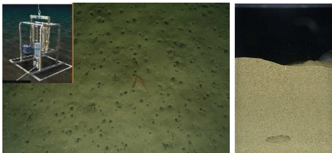
Fig. 1. The SPI system (inset) and example Plan View (left; showing burrow openings on the sediment surface) and SPI (right; showing one intersected burrow segment) photographs.
