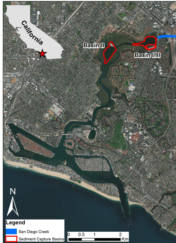
Figure 2: Newport Bay is an urban estuary of southern California where sediment is managed for water quality, wetland habitat, recreation, navigation, and the provision of urban amenities. Dredging focuses on sediment capture basins (Basin II and Basin I/III) and a TMDL was implemented to regulate watershed loads from San Diego Creek (highlighted in blue).
