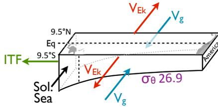
Figure 17: Schematic tropical Pacific box used for the temperature advection calculations (section 6). The red, blue and black arrows indicate the quantities evaluated and are shown in the direction of their mean flow. The ITF (green arrow) could not be evaluated with the data available here, and is treated as a residual.
