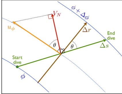
Figure 5: Schematic diagram showing the relations among the vectors  $\Delta s$  (glider motion during a single dive from  $\phi$  to  $\phi + \Delta\phi$ ),  $\Delta r$  (perpendicular to  $\phi$  contours, with angle  $\theta$  from  $\Delta s$ ),  $V_N$  (cross-track transport, perpendicular to  $\Delta s$ ), and the pseudo-velocity  $u_\phi$  (parallel to  $\phi$  contours; section 2.3).
