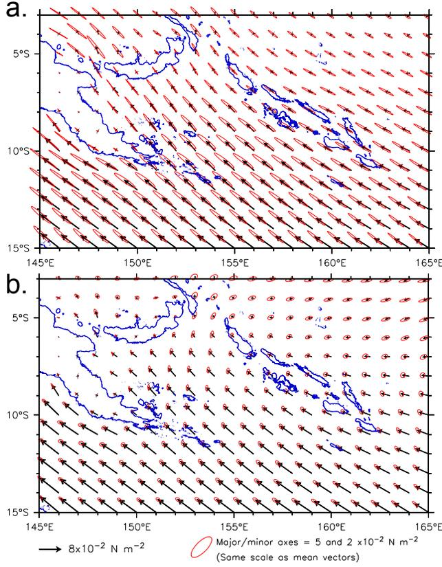
Figure 3: Wind stress variance ellipses for (a) annual cycle and (b) interannual anomalies. Black vectors are means. Both panels use the same scale for vectors (lower left) and ellipses (lower right).
