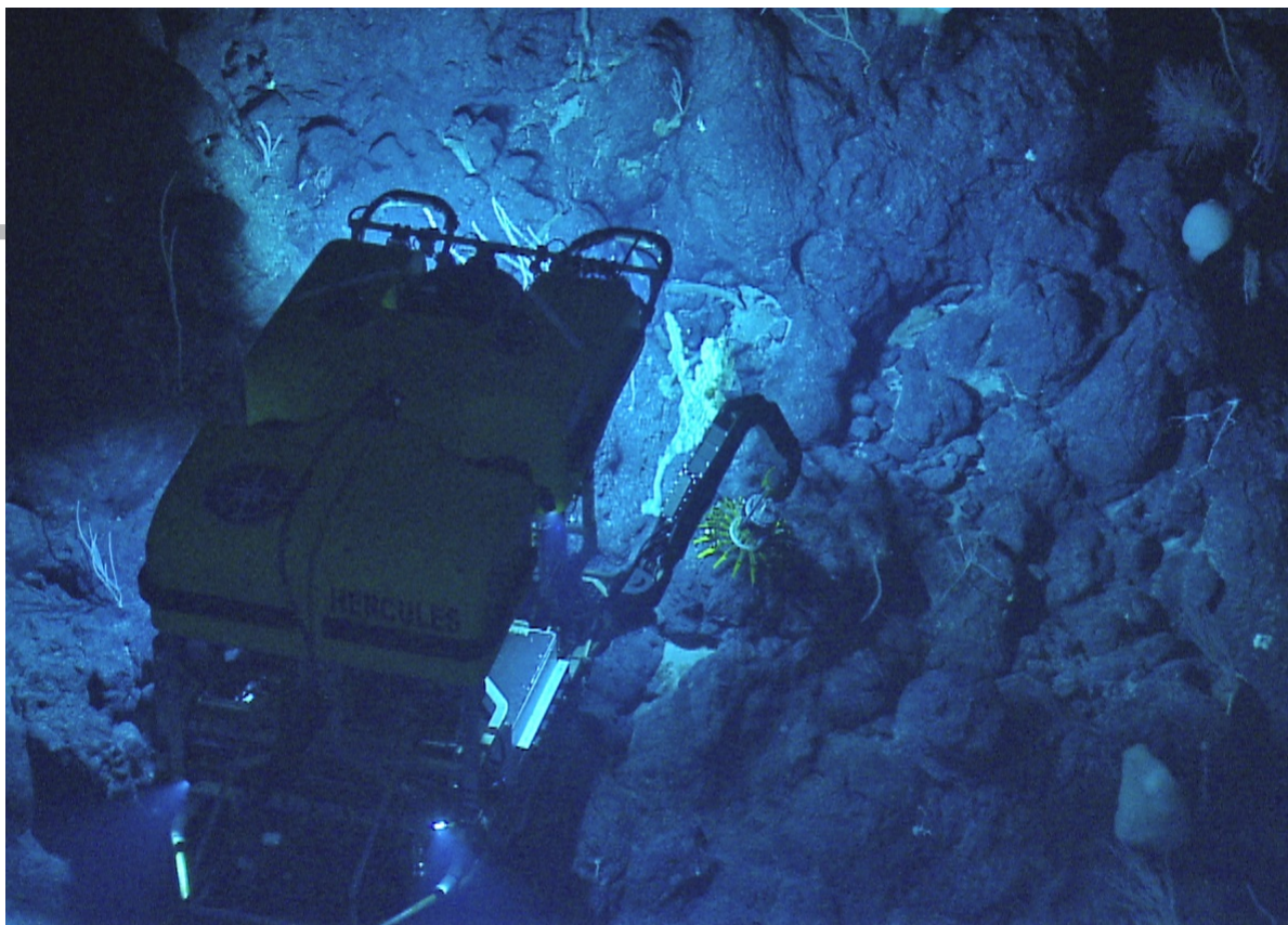
Figure 1: The JPL-Nautilus gripper, located at the end of the robotic arm, anchors the ROV Hercules to exposed rock on a seamount at 2000m depth.
