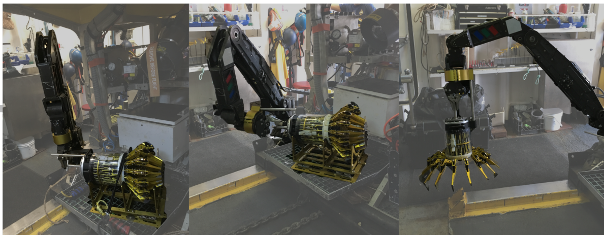
Figure 14: Before deploying the gripper, its integration with and operation by the ROV Hercules was tested on deck. These images show the position of the gripper on the ROV when not in use (left) and how the gripper is picked (center) up and held by the robotic arm (right).
