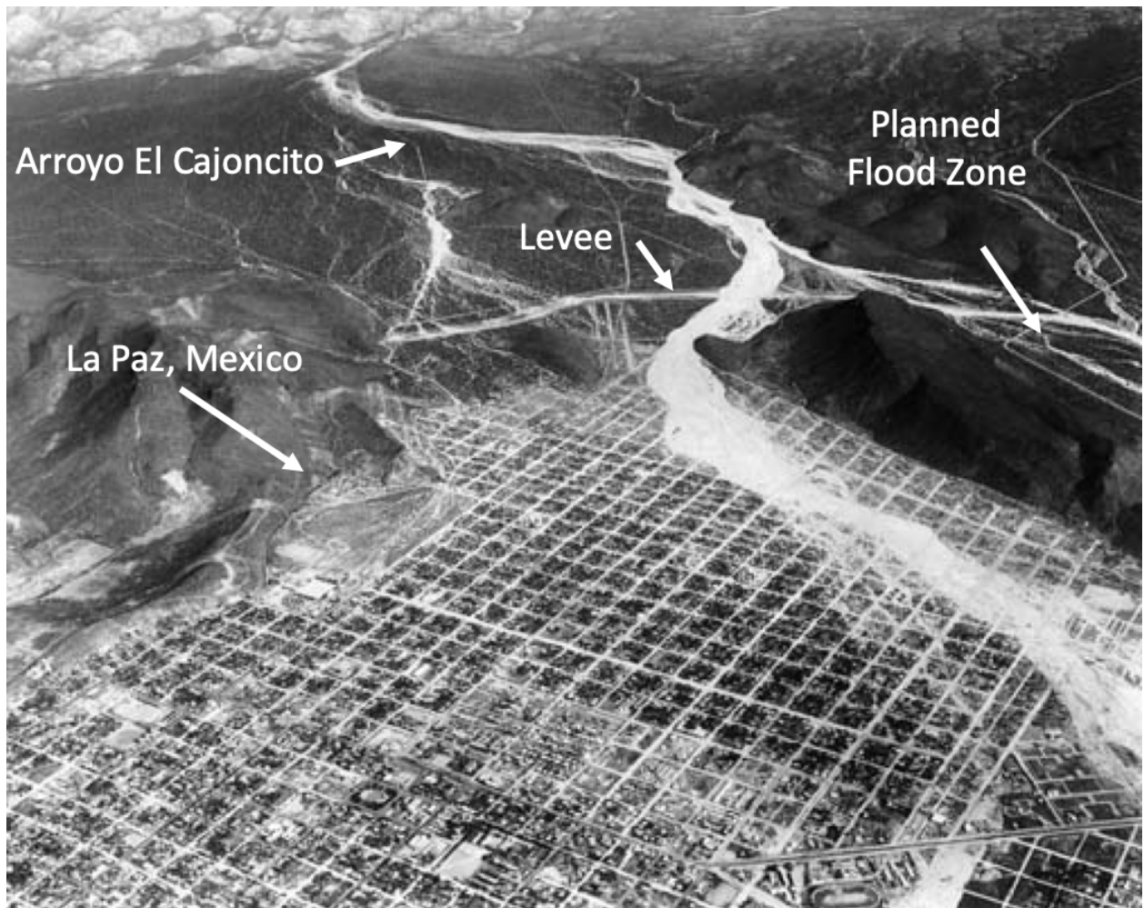
Figure 3. Aerial photo of La Paz, Mexico in October, 1976 after precipitation and runoff from Hurricane Liza caused the Arroyo El Cajoncito to avulse through a protective levee, sending fast moving flood water, mud and debris through an urban development. This event epitomizes ultrahazardous flooding. (Photo by Harry Merrick).
