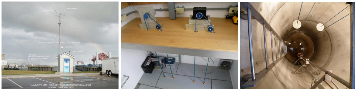
Figure 2 NWLON station at Mackinaw City, MI (courtesy Jeff Oyler, CO-OPS and USACE). Station setup includes numerous antennas including a NOAA CORS Network receiver (left). Inside, measurements are made from the table datum (middle) into the stilling well (right)
