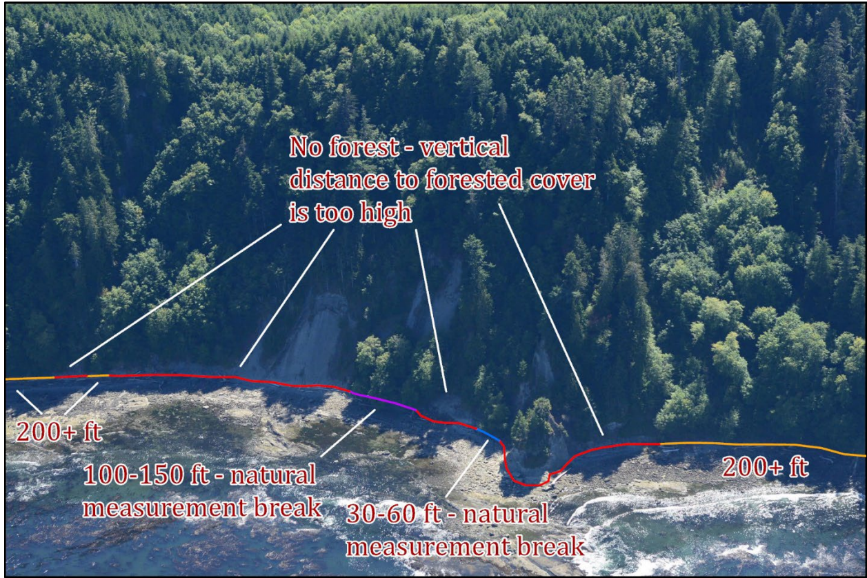
Figure 12. Example of forest width class measurement along No Appreciable Drift - Bedrock shoreform in oblique imagery (DOE 2018). Shoreline sections marked in red are classified as no forest due to the height at which forested cover begins. Shoreline sections marked in blue and purple are classified as 30-60 and 100-150 feet width classes, respectively, as a natural break in forested cover is present. The orange shoreline sections represent measurements of forested cover widths greater than 200 feet.
