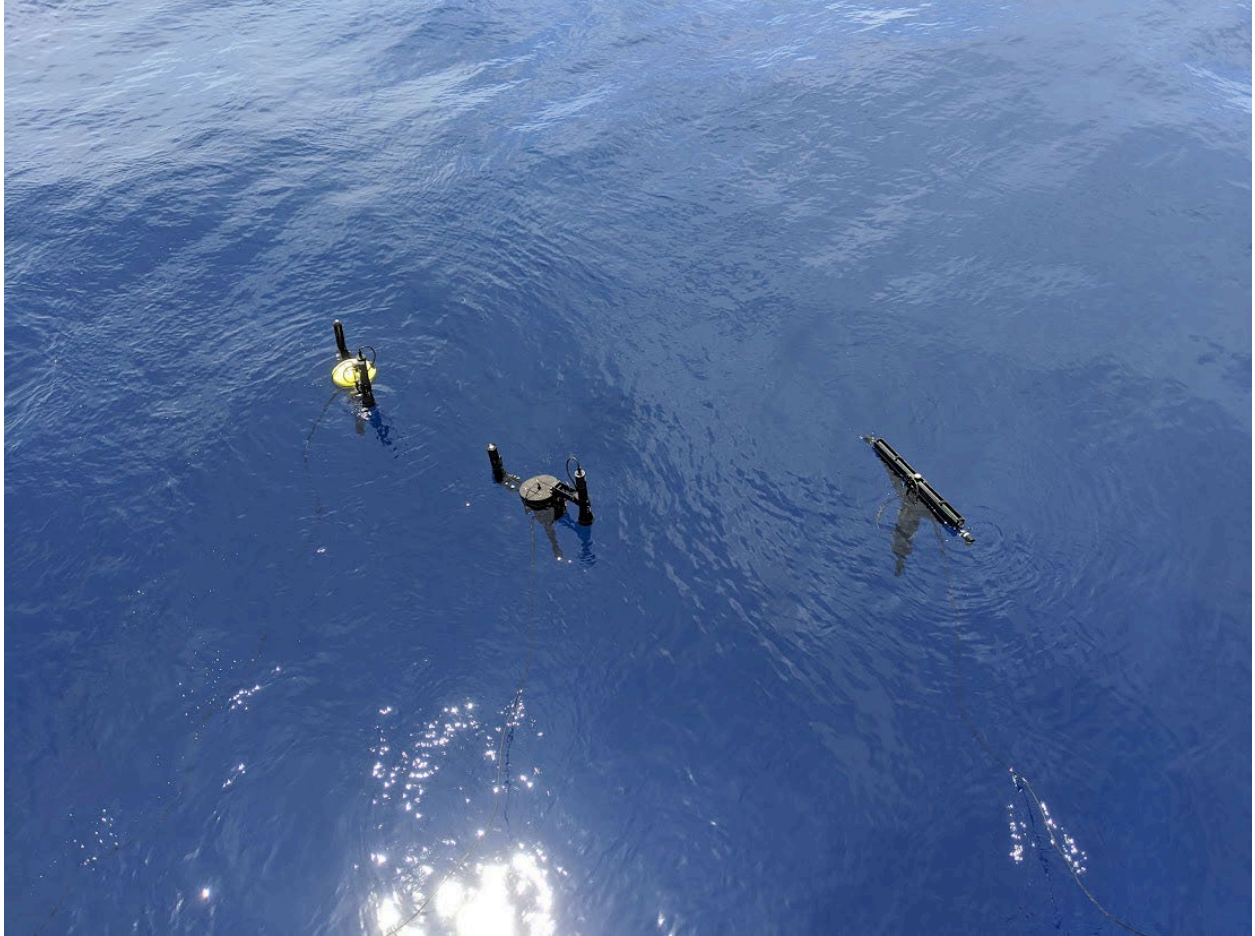
Figure 6. Simultaneous deployment of two SBAs (left and middle) and one HyperNAV (right).
