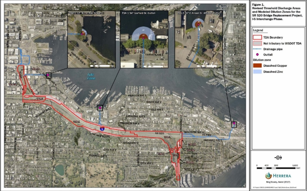
Figure 1. Satellite photograph of the SR 520 Bridge Replacement, I 5 Interchange Phase project site in Seattle, Washington. The insets show the revised threshold discharge areas (TDAs) and modeled dilution zones in Lake Union.
